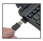
3. Connect the interface cable to the interface port of your computer.
